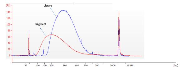
Agilent High Sensitivity DNA trace of samples prepared from NA12878 Coriell DNA, for mean library insert of 350 bp (post-library amplification). Notice, obtaining a mean aligned insert size of 350 bp requires libraries with a peak height of  $\sim$ 560 bp on the Agilent system, due to the broad size distribution of the library and accounting for the adapter length ( $\sim$ 125 bp).
